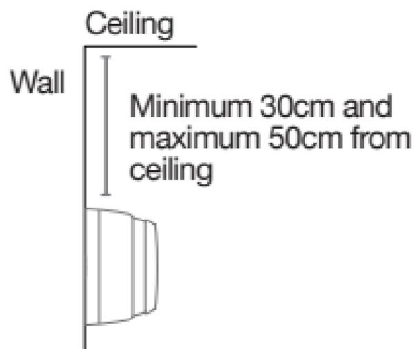
For wall installation; a minimum of 30cm and maximum of 50cm from the ceiling.
