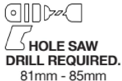
2. Using your hole saw (81mm-85mm), cut a hole into the surface.
