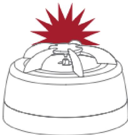
Please note that when the alarms are placed in 'Link Mode' they can't be inserted into the mounting base.
